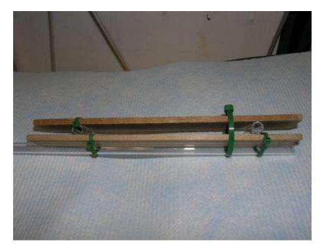
For the fish tests, the stakes would fit in the test containers, so the stakes were submerged in the test solutions by attaching them to glass rods with nylon cable ties (refer to photograph 1). If the glass rods floated, they were weighted down (above the surface of the water) so that the stakes were totally submerged (refer to photograph 2).
